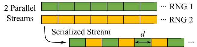
Figure 2. Showing how parallel streams of two independent RNGs can be serialized when run on a serial processor. In the shown case the parallel program operates on equal blocks d of random numbers.
