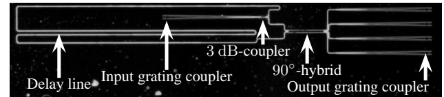
Figure 3. Photograph of an integrated DQPSK receiver in silicon-on-insulator without photodetectors. The footprint is about 250 \mu\text{m} \times 2000 \mu\text{m} , mainly due to the delay line and the 500 \mu\text{m} long tapers between the grating couplers and single-mode waveguides. Smaller footprints can be achieved with focusing grating couplers and meander-shaped delay lines.
